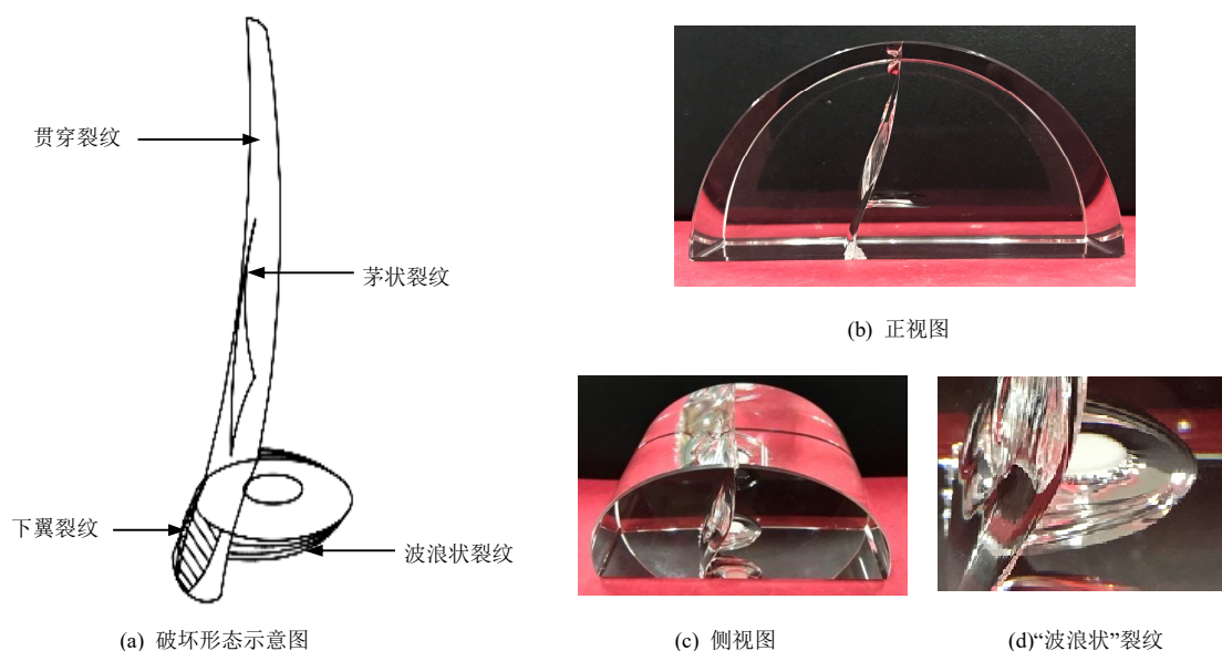
图 11 试样破坏形态 Fig.11 Sample failure modes
